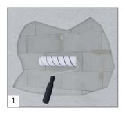
Clean the surfaces underneath before starting processing and prepare them with deep-penetrating primer or adhesive and bonding primer.
