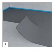
Apply a perimeter isolation strip all around. Even out any rough unevenness before tiling. It can be cut simply using a carpet cutter.
