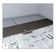
The floor covering can be installed after curing of the thinbed mortar. Then, the joint area must be sealed using the wedi Tools sealing tape as well as a sealant.
