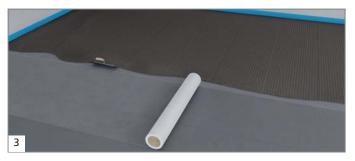
The entire board surface area is then reinforced with wedi Tools reinforcement tape and fixed in place in a layer of tile adhesive, making it ready for tiling. Alternatively, in wet areas, the seal can also be carried out with wedi 610 or wedi Tools sealing tape.
